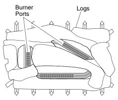
Figure 18 - Installing Log set (Top View)
